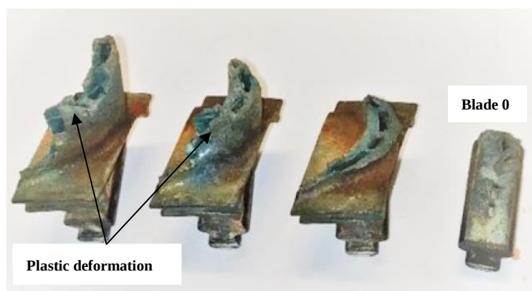
Figure 2. Blade 0 and several blades affected by the impact with the fragment of blade 0
