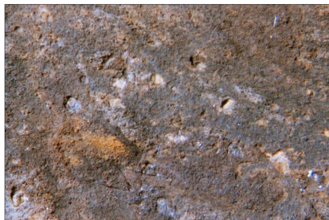
Figure 4 Macroscopic observation on the internal pipe surface shows pitting corrosion (magnification of 50x)
