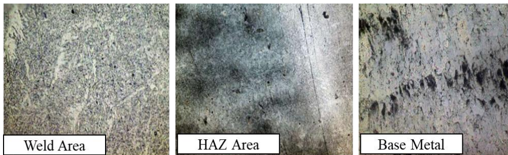
Fig. 17 In-situ Metallography Result After Repair
