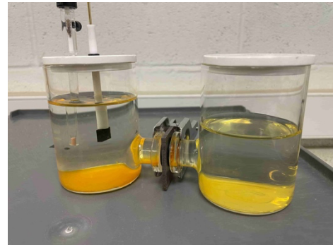
Figure 1 - Double Exposure of 3mm Cast Iron Working Electrode
