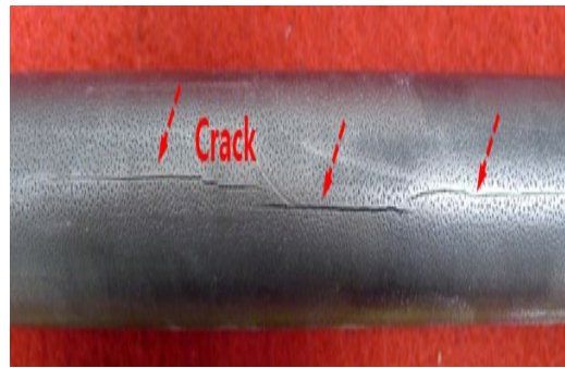
Figure 1: The macro-optical image of the failed tube shows the longitudinal cracks.
