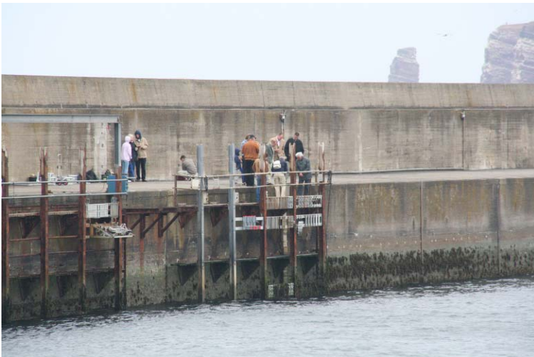
Figure 15. Exposure tests in seawater of the island Helgoland within a research project supervised by the University of Stuttgart
